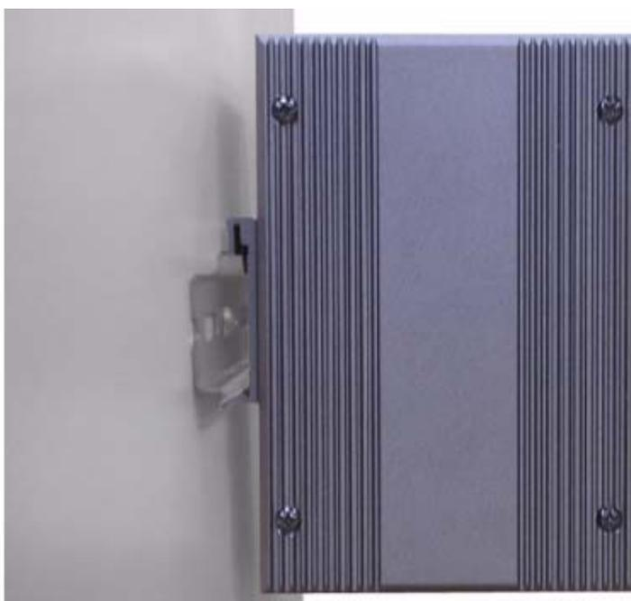
**Figure 2.31 DIN-rail Step 2**
